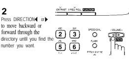
→ Pressing ➤ allows you to search forward through the memory in Speed Dial number order (from 01 to 30) and **◄** allows you to search in reverse order.
